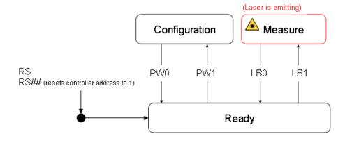
When powering the CONEX-LDS, the controller starts initialization. When initialization is successful, the controller goes to the READY state. The controller can go to the CONFIGURATION state using the PW1 command. In the CONFIGURATION state, the CONEX-LDS allows changes to all configuration parameters, like gains or controller address. The PW0 command saves all changes to the controller's memory and returns the controller back to the READY state.
