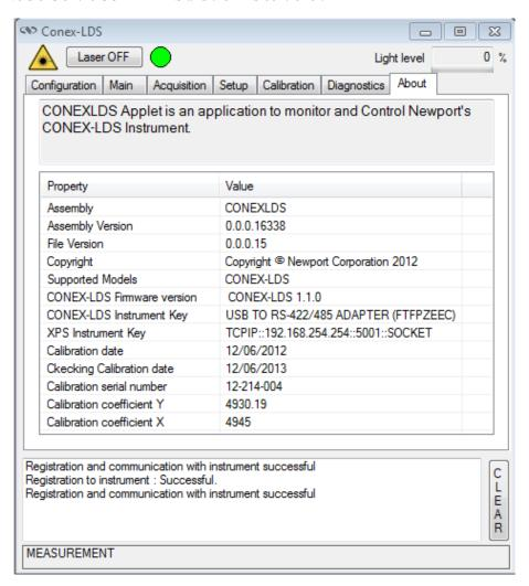
For an external data logger, refere to the analog out pinouts and the gains table to convert from voltage to position. Refer to the CONEX-LDS Users manual for more information.
